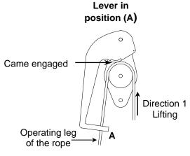
Lever in position (A): direction 2 blocked & direction 1 free
